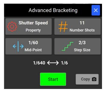
sequence. The step size sets the number of steps to adjust the exposure between each shot. The number of shots specifies the number of shots in the sequence. The maximum number of shots is dynamically calculated based on the mid-point and the possible camera values. Clicking the Copy button will set the mid-point to the camera's current value.
