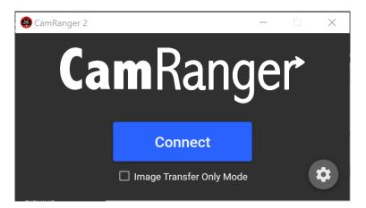
The connection screen appears after launching the application. In addition to the large "Connect" button, there is an "Image Transfer Only Mode" check box and a button to open the application preferences. The preferences can also be accessed from the menu bar. The default mode is to have Image Transfer Only turned off. If this box is checked, images will automatically be transferred as they are captured. However, all controls and image display will be removed.
