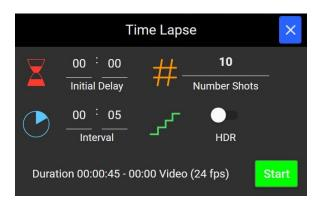
The Timer tab is accessed by pressing the stopwatch button and is used to configure the CamRanger as an intervalometer as well as to specify exposure times when the camera is bulb mode.
