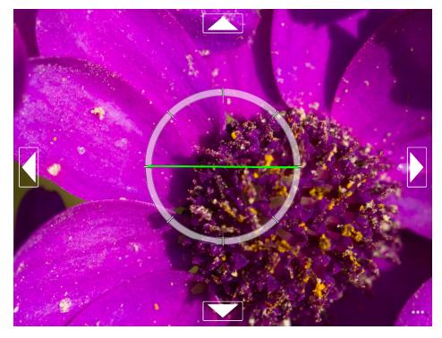
Double clicking on the image during live view will zoom in at that point, and then alternatively zoom back out. When zoomed in, arrow buttons will appear at the edges enabling small adjustments to the zoom positioning.
