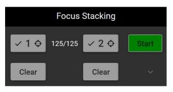
A new focus stacking method is available which automates more of the process. Changing to the previous focus stacking method is still possible by turning on "Classic Focus Stacking" in the settings. The new focus stacking method requires the user to specify the nearest and furthest focus positions and
