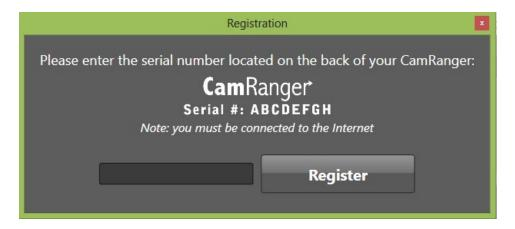
Enter the 8-character CamRanger serial number. The serial number is located both on the bottom of the back cover as well as above the battery underneath the back cover. Note: the serial number contains only letters and NO numbers.
