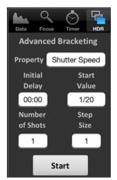
The "HDR", or Advanced Bracketing, tab can be used to generate a series of photos with varying exposures.
