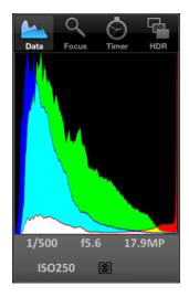
The data tab shows an RGB histogram and meta-data associated with the image in the main image view. The following meta-data is provided:
