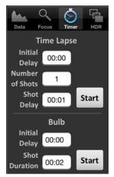
The timer tab allows the use of the CamRanger as an intervalometer as well as specifying exposure times when the camera is in bulb mode.
