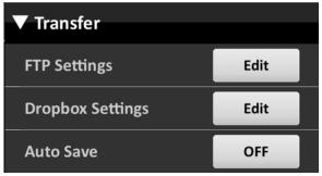
Name, Username, Password is entered, the user can test the connection. Optionally a remote directory can be specified. This directory must already exist or be created with the "Create" button. The user must be bridged into an existing wifi network or have access to cellular data to share images to an FTP server.
