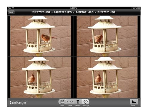
The images displayed within the compare screen are not full resolution, but are scaled down. They can be zoomed in and out with a double tap or pinch zooming. To save, delete, or rate an individual picture, first tap the image to select it, as indicated by a yellow outline around the image.
