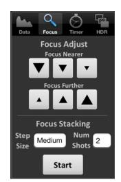
The focus tab is only enabled during live view and provides advanced focusing controls.
