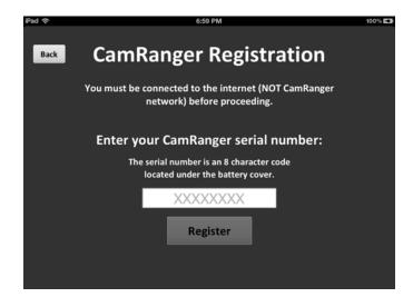
Enter the 8-character CamRanger serial number. The serial number is located both on the bottom of the back cover as well as above the battery underneath the back cover. Note: the serial number contains only letters and NO numbers.
